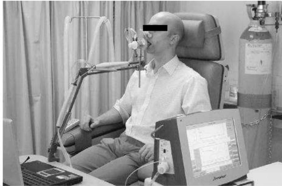
**Figure 2** Subject performing a washout. The supply of wash-in gas (0.2% SF<sub>6</sub> in air) is provided by the cylinder in the background. An Innocor™ gas analyser is used to measure flow and SF<sub>6</sub> concentration and expiratory volume is displayed to the subject on a separate screen.
