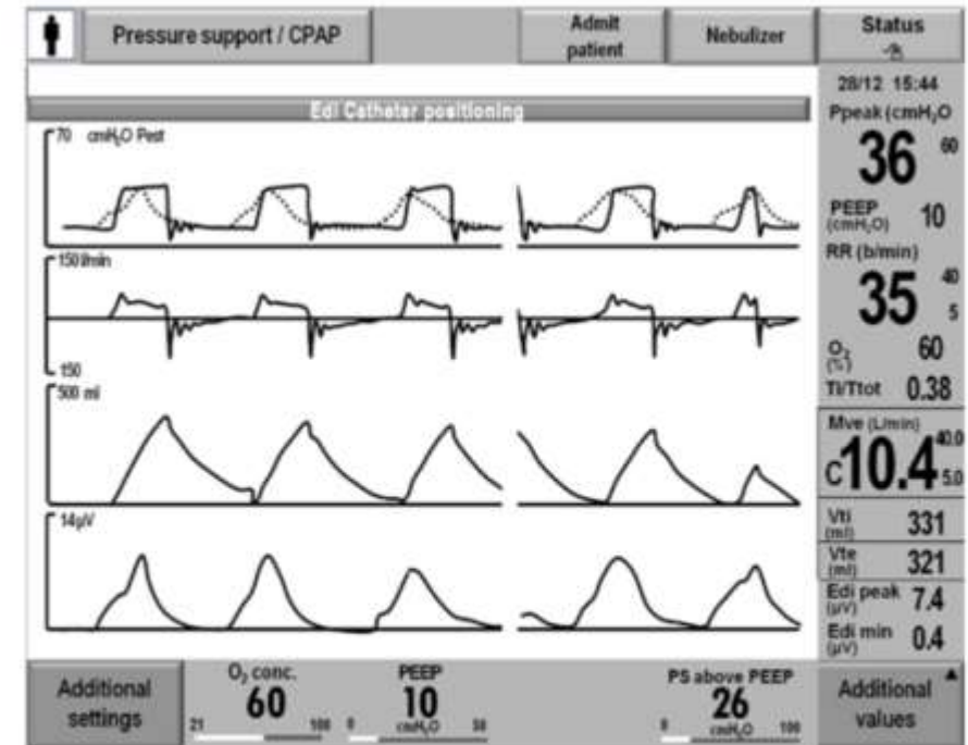
Figure 3: A drawing of the main screen of the SERVOi ventilator. This represents an adult patient in pressure support/CPAP mode. The top waveform is the pressure/time waveform (solid) and the Edi waveform (dashed line). The second waveform is flow/time, the third is volume/time and the fourth (bottom) is Edi/time. Note that the Edi signal from the diaphragm and the pressure waveform from the ventilator do not correspond. This is an example of patient-ventilator asynchrony (See text for further description).
