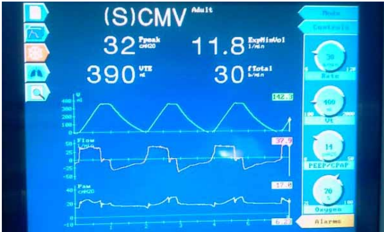
Patient of ARDS being ventilated using ARDS Network strategy (Tidal volume = 6 ml/kg, Body weight = 66 kg)
