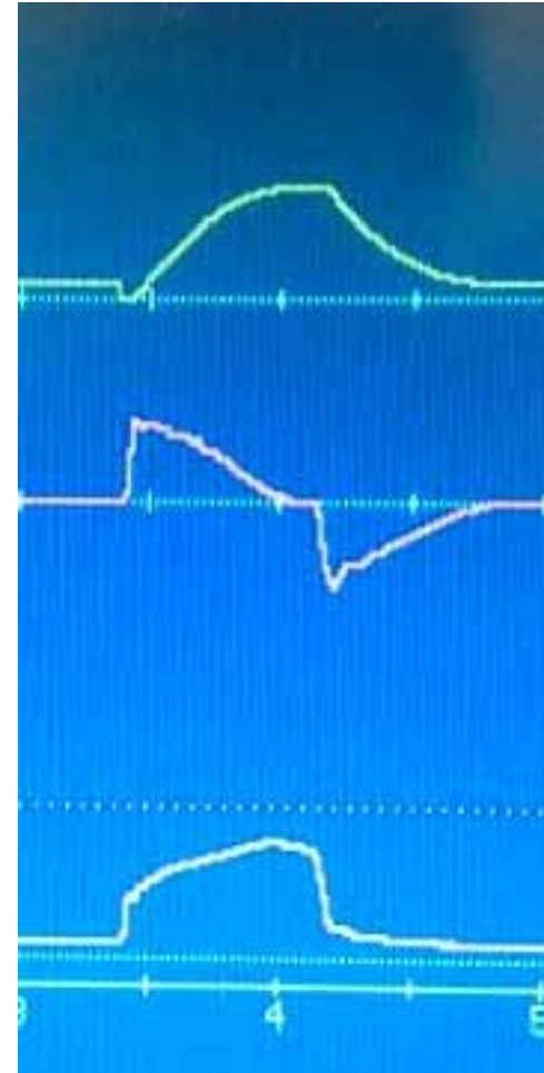
DESCENDING RAMP FLOW
