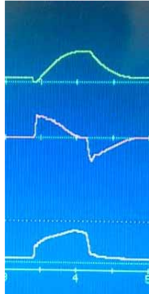
DESCENDING RAMP FLOW
