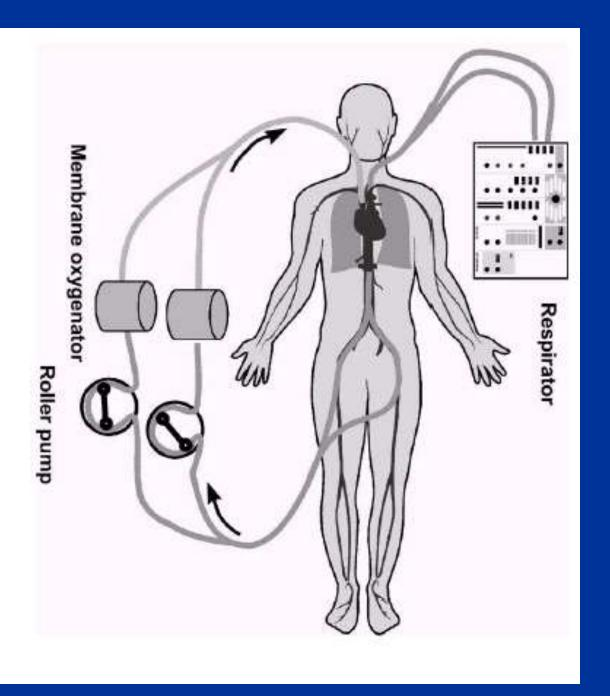
Schematic drawing of a low-flow venovenous ECMO circuit.
